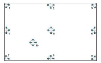
The more points used for calibration, the greater the accuracy. Errors in calibration may occur due to viewing angle, or individual skill, and there may be little difference in using 16 or 25 points. Note that a stylus is recommended for the most accurate results.
