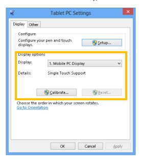
The inbox calibration process prompts for clicking on the 16 points located in the four corners of the screen. If clicking on wrong places, please use the Press and hold on a certain point will return to the previous position.
