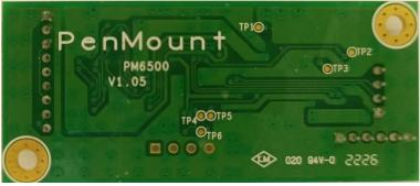
PM6500C8 supports 4/8 wires touch panel, R14 is mounted in the circuit.
