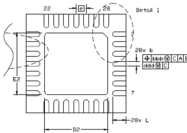
Fig. 4: QFN-28 Package Drawings - Bottom View
