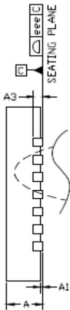
Fig. 3: QFN-28 Package Drawings – Side View
