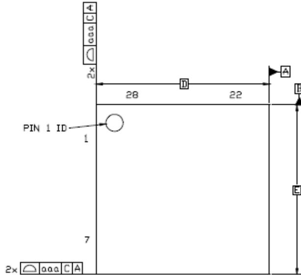
Fig. 2: QFN-28 Package Drawings - Top View
