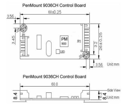
**Mechanical Size** : PM9036CH5 and PM9036CH8 are the same mechanical size.
