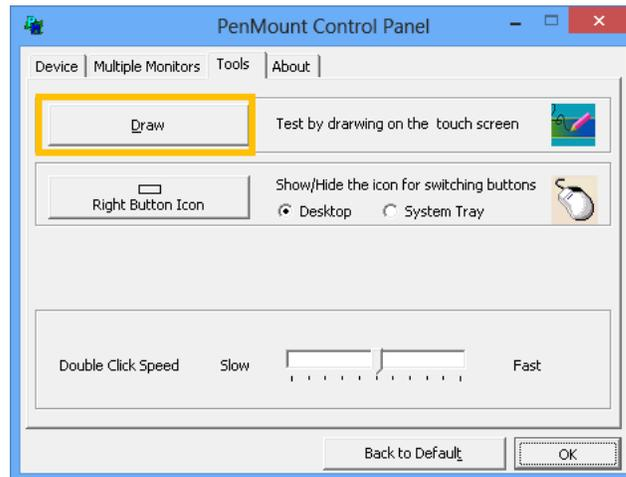
Touch the screen with your finger or a stylus and the drawing screen registers touch activity such left down, left up, right down and right up.
