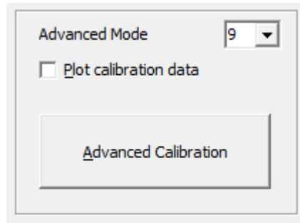
The advanced calibration supports 9, 16 or 25 point modes. Please scroll down the “Advanced Mode” drop down list for choosing a desired mode.
